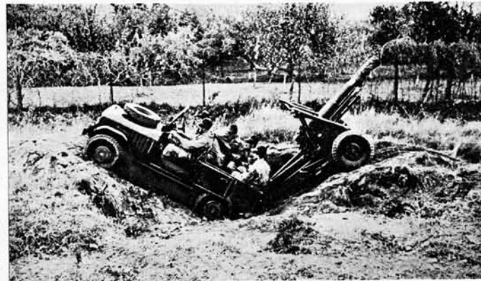
Above: The Gunners may soon be getting this portable Italian 105 mm howitzer shown here undergoing tests in Italy. It can be dismantled and carried by mulepack, flown in three sections by helicopter, or broken down into 30 parts and manhandled.
