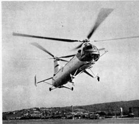
The Army's new helicopter: the twin-engine Bristol 192. It can carry 25 armed troops and be used for paratrooping, supply dropping and as an ambulance.
