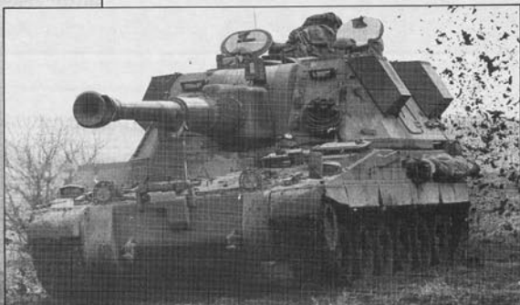
AS90 kicks up the dirt during a mobility demonstration on Salisbury Plain. It has an official top speed of 53 kmh
