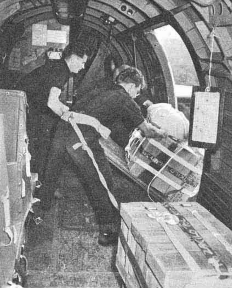
On a signal from the cockpit the despatchers lift up the board and a pack slides out into the slipstream. Note the long-lead belts and manifest. Track suits allow the despatchers to move freely and safely in the plane.
