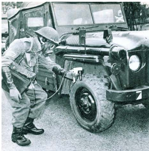
A Land Rover suspected of carrying radio-active dust is checked by a contamination meter. A Geiger counter measures the amount of infection.
