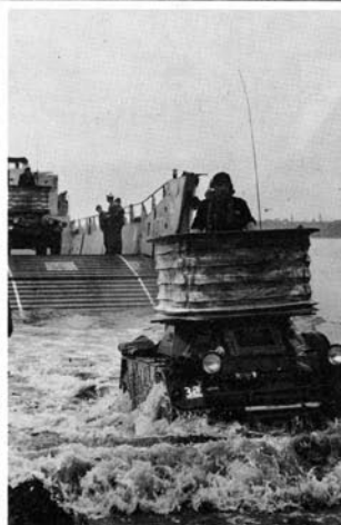
Top: A chopper from Fearless picks up invasion troops on the deck of Sir Tristram. Above: Ferrets of 3rd Royal Tank Regiment splash ashore complete with waterproofing "mini-skirts." Left: A medium wheeled tractor laying assault tracking.
